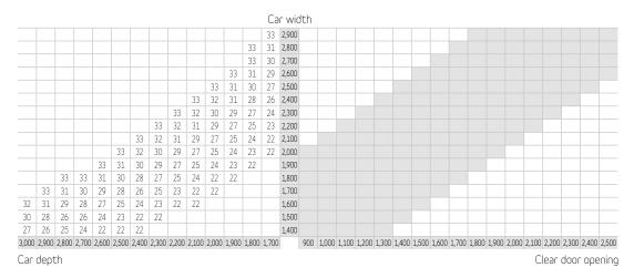
Note: Car width and depth variable in increments of 5 mm. For simplification, table samples show increments of 100 mm.
