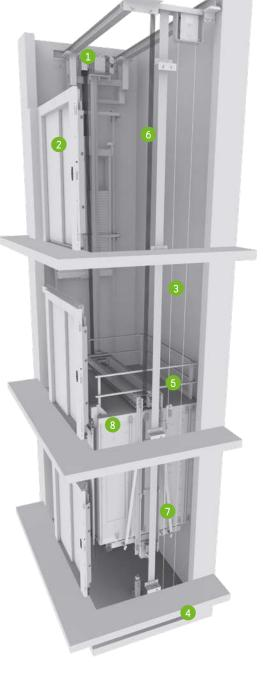
1 DRIVE Compact, quiet, gearless, energy efficient, speed regulated (VVVF) permanent magnet electric motor.
